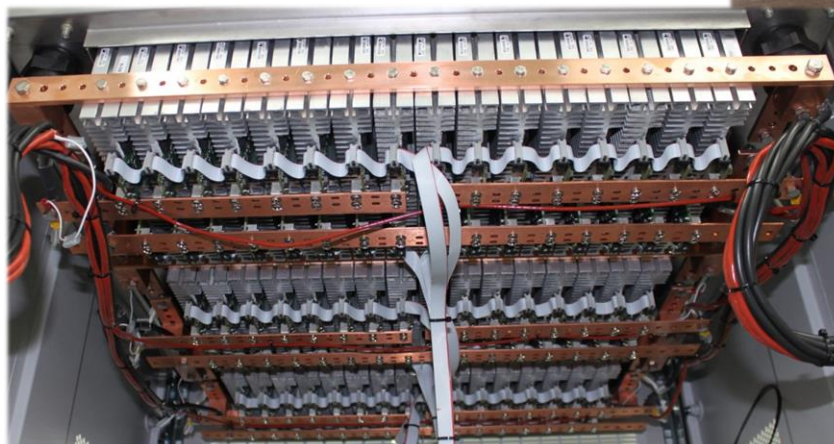
Example of a power bloc manufactured with more than 1000 transistors
